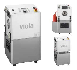
The portable, high performance viola high-voltage testing and diagnostics device is available in two different configurations. The standard variant is used for cable and cable sheath testing of electrical equipment and medium-voltage cables up to 35 kV. Another function is insulation testing on electrical equipment. The patented VLF-truesinus<sup>®</sup> technology (0.1 Hz sine voltage) guarantees a high level of measurement accuracy.
