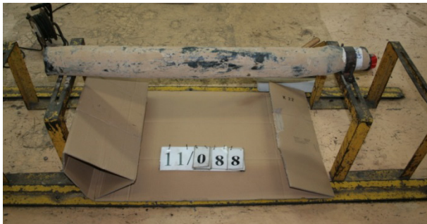
Rusty noted inside wraparound recovered from site
