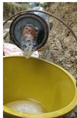
Figure 40 Incomplete degassing of the cable in the factory, after 14month in operation
