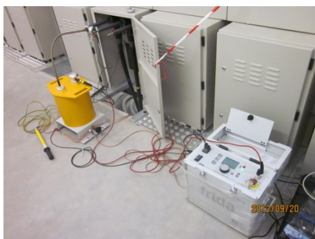
Figure 89 Portable on-site PD detector with PD location (BAUR PD portable)
