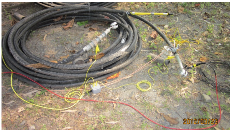
Figure 64, connection arrangement with guard ring and corona hoods, VSE box, Frida TD connection
