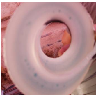
Figure 41 Aged XLPE insulation, voids in XLPE, 115kV cable
