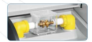
Determining the breakdown voltage
