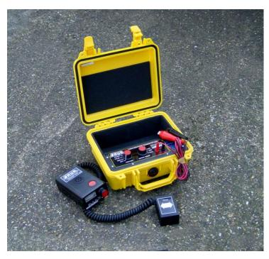
large size push button energises the receiver and ensures that it cannot inadvertently be left on.
