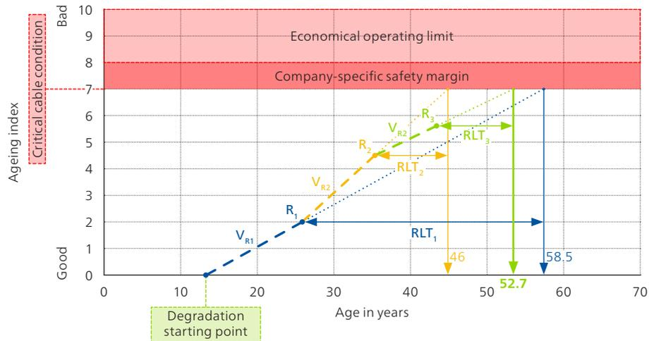
An initial dissipation factor measurement after a duty period (DP) of 26 years gives a value for the ageing index  $R_1$  of the cable of 2.0. The speed of ageing  $V_{R1}$  can thus be calculated after the first measurement. With the speed of ageing, the statistical remaining life time (RLT) of the cable can be calculated after the first measurement.
