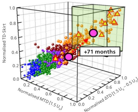
3D illustration of the correlation between normalised evaluation parameters of dissipation factor measurements MTD,  $\Delta$ TD and TD-Skirt: The framed area top right in the illustration exhibits a high probability of error.
