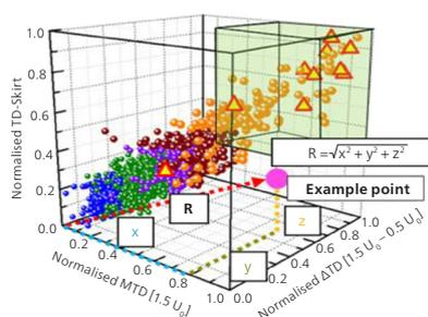
Following on from the subsequent measurement and the recalculation of the ageing index R, and based on the index R of the two measurements, the speed of ageing and the anticipated remaining life time of the cable route are calculated. The difference between the economical operating limit and the specific safety margin of the utility company makes it possible to conclude when work will be required on the cable route.
