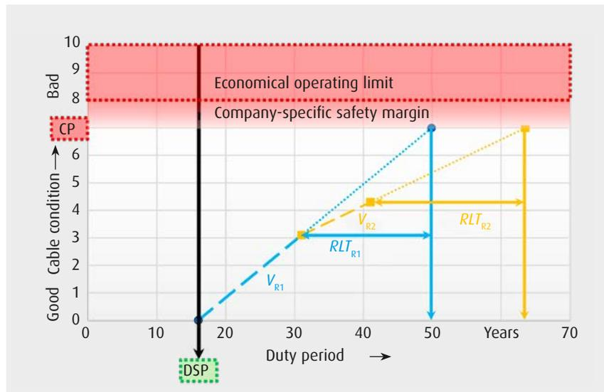
Figure 6: statex recalculates the remaining life time when repeat measurements are performed.
