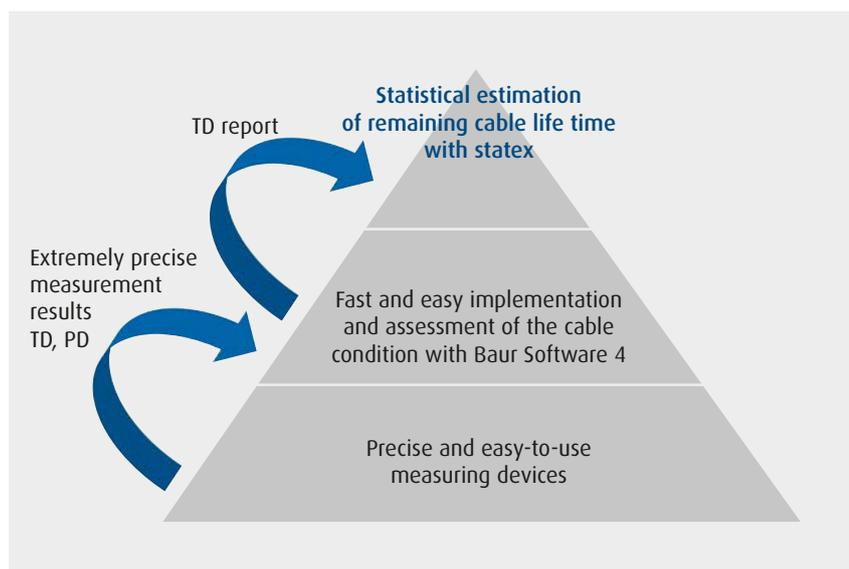
Figure 3: With the new statex software, the values from the dissipation factor measurement can be used to predict the remaining life time of medium-voltage cables.
