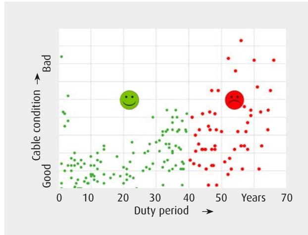
Figure 1: A strategy for replacing cables based on absolute age would mean that many cables that are still intact (as illustrated in the bottom right area of the diagram) would be replaced.
