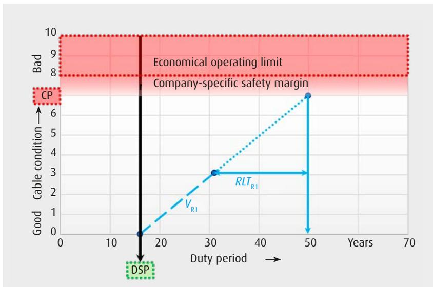
Figure 5: The statex software can use the  $\tan \delta$  measured values to calculate the ageing index and estimate the remaining life time of the cable.
