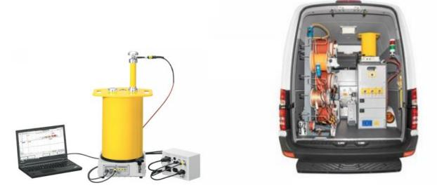
The small and lightweight PD-TaD 80 (shown on the left with Power Box and notebook) also fits in beautifully in small cable test vans with a maximum weight of 3.5 tonnes.
