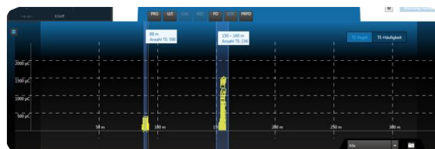
Figure 13 PD localization graph indicating PD activities in 2 locations
