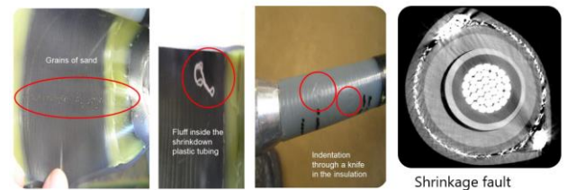
Figure 10 Post-mortem of joints with PD activities
