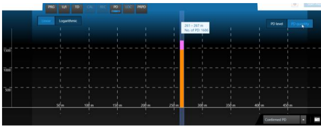
Figure 7 PD activity (quantity per time unit) at transition joint
