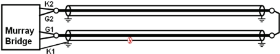
Fig.6. Murray Bridge connection diagram
