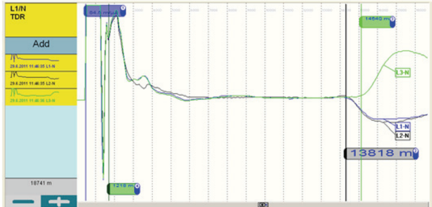
Fig.3. TDR trace of an AC submarine cable, Italy Main Land -Ischia [2]
