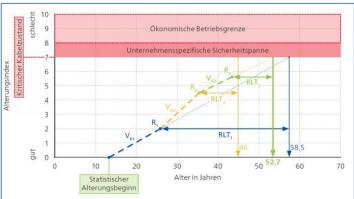
The statex® pro software calculates the expected remaining life time based upon tan  $\delta$  at 1.5 U<sub>0</sub>, the difference between tan  $\delta$  (1.5 U<sub>0</sub>) and tan  $\delta$  (0.5 U<sub>0</sub>), and TD-Skirt, as well as statistical calculations based on a data pool. TD-Skirt indicates trends or fluctuations of tan  $\delta$  over multiple measurements.
