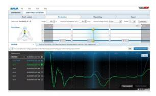
The Smart Cable Fault Location Guide speeds up cable fault pre-location and pin-pointing. The software can also be linked to the BAUR cable database and a geographical information system to narrow down the type and location of the fault even more rapidly. BAUR software helps during pin-pointing, too, and even protects the cable: The BAUR app shows the location of the fault on the display and allows the surge current generator to be remotely
