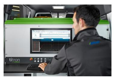
interface and quickly obtain reliable results. However, the software also offers an expert mode in which experienced measurement engineers have direct control over processes and parameters. Help is also at hand for users whilst locating faults, with cable data and measured values linked to maps so that operators can quickly see where the problem lies.
