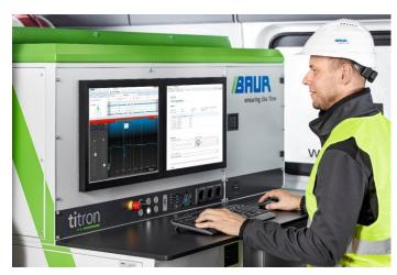
Parallelised processes – such as the combination of dissipation factor and partial discharge measurement into a single sequence – speed up measurement tasks. Measurement engineers are thus able to collect significantly more information and generate additional benefits for asset and maintenance management. To get the most out of the information, standard processes can be augmented by the definition of custom templates
