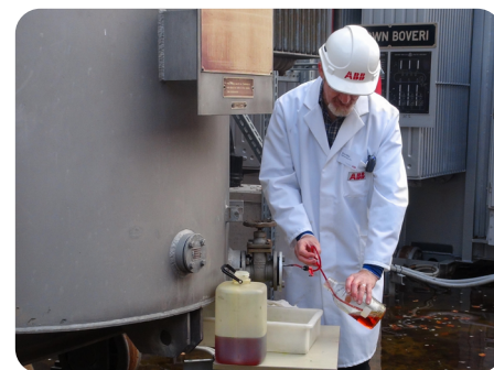
Eric Killer from ABB Sécheron AG (left - during sampling, above - in the laboratory) uses BAUR devices to determine the breakdown strength of the insulating oil as well as the laboratory values that allow conclusions to be drawn regarding the oil condition.
