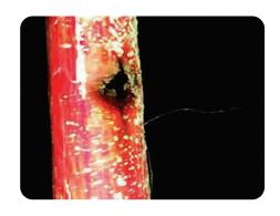
pin-pointing set (UL 30 and BM 30) it was possible to confirm the graphical evaluation just a few minutes later and the team from Advanced Vision was able to locate the fault immediately and rectify it quickly.
