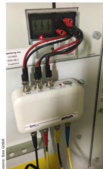
Figure 1: Connection of the partial discharge measuring device to the switchgear VDS sockets of a wind farm
