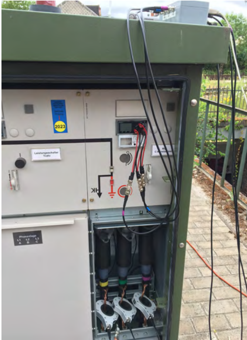
Figure 3: To compare the measurement quality, the liona partial discharge measuring device was connected to both the new VDS PD coupler (top) and HFCT sensors (bottom).
