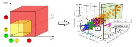
Following on from the subsequent measurement and the recalculation of the ageing index R, and based on the index R of the two measurements, the speed of ageing and the anticipated remaining life time of the cable route are calculated. The difference between the economical operating limit and the specific safety margin of the utility company makes it possible to conclude when work will be required on the cable route.
