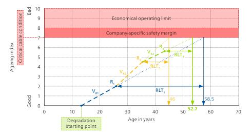
An initial dissipation factor measurement after a duty period (DP) of 26 years gives a value for the ageing index  $R_1$  of the cable of 2.0. The speed of ageing  $V_{R1}$  can thus be calculated after the first measurement. With the speed of ageing, the statistical remaining life time (RLT) of the cable can be calculated after the first measurement.
