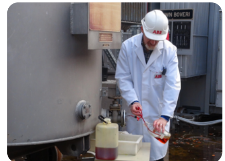
Eric Killer from ABB Sécheron AG uses BAUR devices to determine the electric strength of the insulating oil as well as the laboratory values that allow conclusions to be drawn regarding the oil condition.
