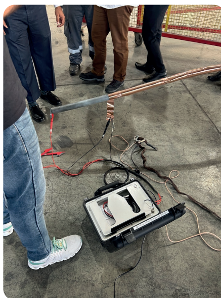
Step TDR is perfectly suitable for the cable end
