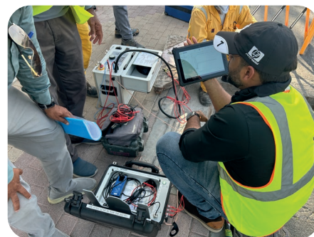
Exact fault location thanks to Step TDR
