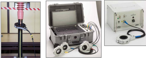
Figure 1 PD online spot testing equipment
