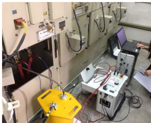
Figure 14 VLF TD PD MWT, frida - VLF offline diagnostic setup
