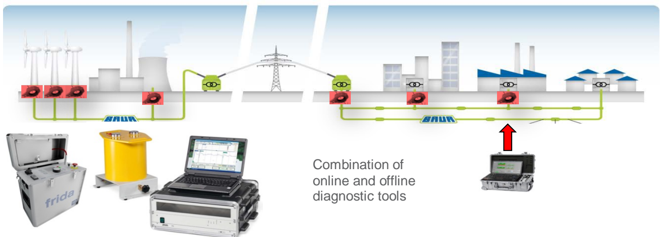
Figure 14 VLF TD PD MWT, frida - VLF offline diagnostic setup
