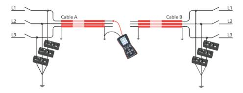
Additional signal injectors can be purchased optionally to determine the conductors of up to ten three-phase cables.
