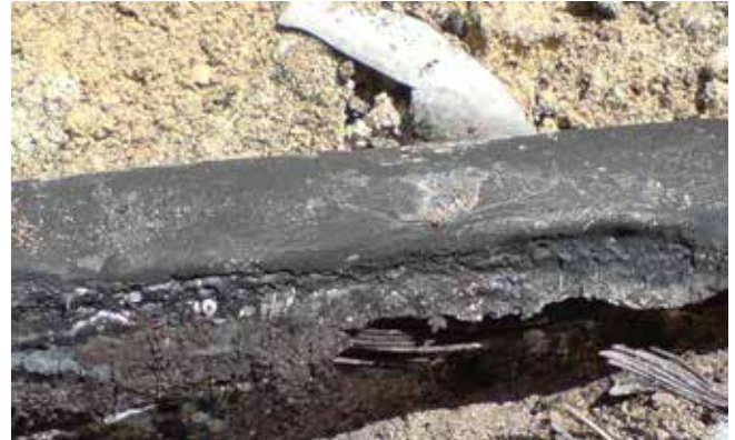
➤ vaporized core after cable fault, 132 kV XLPE
