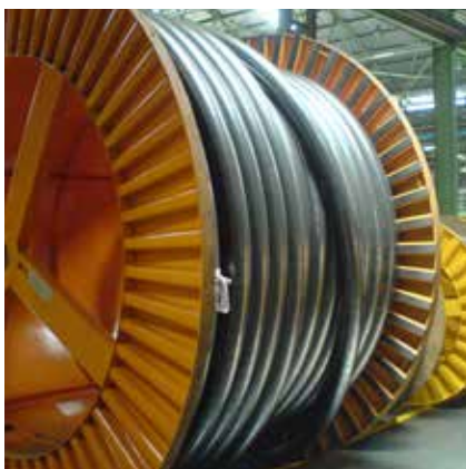
➤ Cable on drum, 115kV single core
