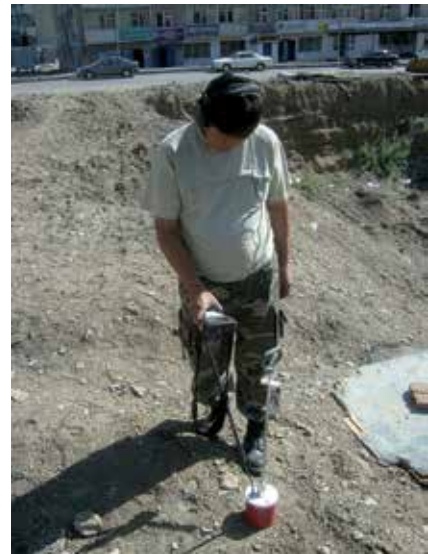
➤ field application acoustic fault location
