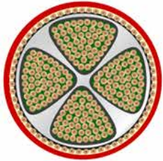
➤ Shielded segmented low voltage cable 3 or 4 conductors plus shield, faults mostly internally.
